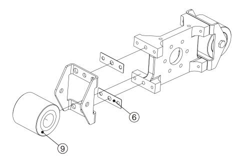
The shims are installed from factory to work at the work conditions indicated (in function of the speed and the work pressure), and following the next tables. **NOTE:** If not indicated on original order, the pumps are factory set to 60 psi.
