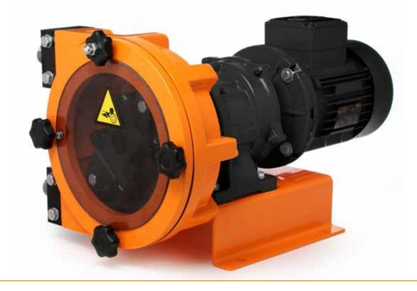
The **DULCOFLEX DFB** is a versatile peristaltic pump, which incorporates both hose and tubing technology. The unique roller design offers a lubricant-free housing unlike typical shoe pumps. With pressures up to **116 psi** and flow rates to **337 gph**, the DFB is a great choice for pumping difficult fluids such as slurries and abrasive chemicals.
