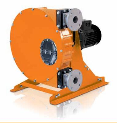
The **DULCOFLEX DFD** is a hose pump designed for pressures up to **232 psi** and flow rates up to **160 gpm**. The unique shoe design is made of steel for smoother and cooler compression. The DFD uses safe **DulcoLube** oil for the shoe lubrication. With suction lifts up to **29 feet**, the DULCOFLEX DFD is a great choice for difficult pumping applications.
