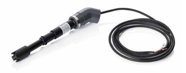
The measured variable "dissolved oxygen" indicates the volume of gaseous oxygen physically dissolved in the aqueous phase in ppm (mg/l) or the oxygen saturation of water in percent. The **DO 3 sensor** is based on visual measurement of fluorescence and can be connected to the process in an immersion pipe or in a flow fitting. It can be used to monitor water rich in oxygen, such as surface water, potable water, as well as for the control of the aeration of aeration tanks in clarification plants.
