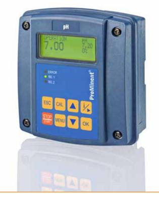
The **ProMinent® DULCOMETER Compact** analyzer provides precise measurement and control of pH, ORP or Conductivity process variables. The pre-configured Compact can be programmed for either pH, ORP or Conductivity control without having to purchase a separate analyzer. Temperature compensation for pH can be added using an optional PT 1000 sensor. The Compact comes standard with pulse relay for pump control, configurable analog output and configurable power relay.
