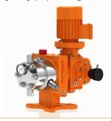
The **ProMinent® Evolution 1** meets the most exacting safety requirements as an extremely robust hydraulic diaphragm metering pump. It stands out thanks to its PTFE multi-layer diaphragm with integral diaphragm rupture warning system and unique diaphragm position control. Its modular construction offers excellent flexibility for countless applications.
