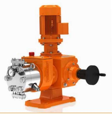
The **ProMinent**<sup>®</sup> **Evolution 3** meets the most exacting safety requirements as an extremely robust hydraulic diaphragm metering pump. It stands out thanks to its PTFE multi-layer diaphragm with integral diaphragm rupture warning system and unique diaphragm position control. Its modular construction offers excellent flexibility for countless applications.
