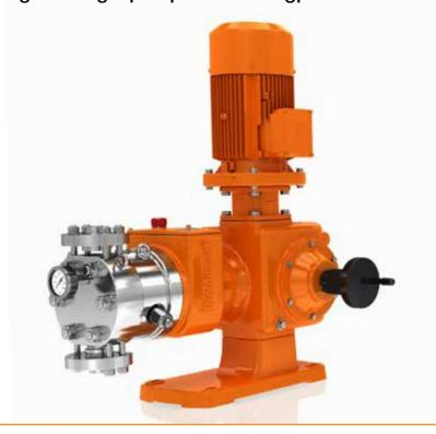
The **ProMinent®** Evolution 4 meets the most exacting safety requirements as an extremely robust hydraulic diaphragm metering pump. It stands out thanks to its PTFE multi-layer diaphragm with integral diaphragm rupture warning system and unique diaphragm position control. Its modular construction offers excellent flexibility for countless applications.
