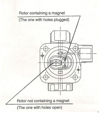
As chemical passes through the gear box, the gears rotate. The epoxy enclosed sensor reads the magnet loaded in the gear for each milliliter of chemical. The electronics stay clean and dry separated from the process liquid.
