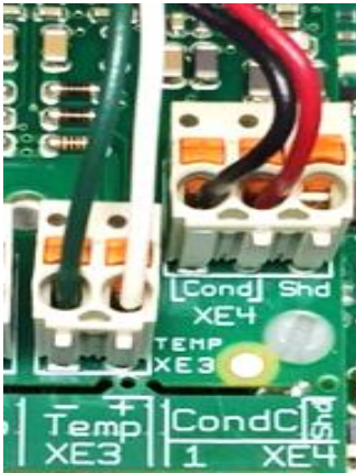
Figure 43 Four Wire Conductivity - Temperature Probe On channel 2
