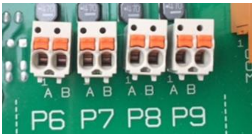
Figure 29A Digital DC outputs 6-9
