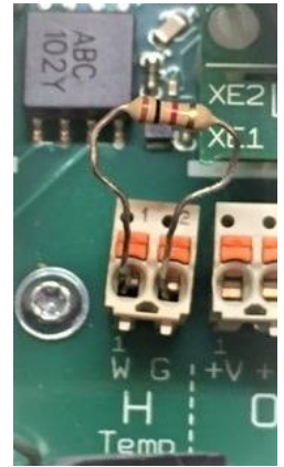
Figure 33 Input H with test resistor
