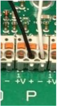
Figure 34 Digital Input wiring
