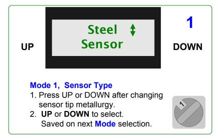
The LogR is set for the tip metallurgy ordered with the LogR. If you change the tip metallurgy, use Mode 1 to select the tip metal or alloy.
