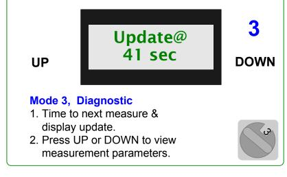
**Update**@ counts down to next corrosion rate measurement.
