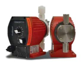
The **ProMinent® Concept** and **beta®** pumps are (Hearty) solenoid metering pumps suitable for Oil & Gas production services. Feed rate is determined by stroke length and stroke frequency adjustments. Stroke length can be adjusted in 10% increments from 10-100%. Stroke length is adjusted from 0-100% with a 4:1 turndown ratio in the **Concept** and 10:1 with the **beta®** pump.
