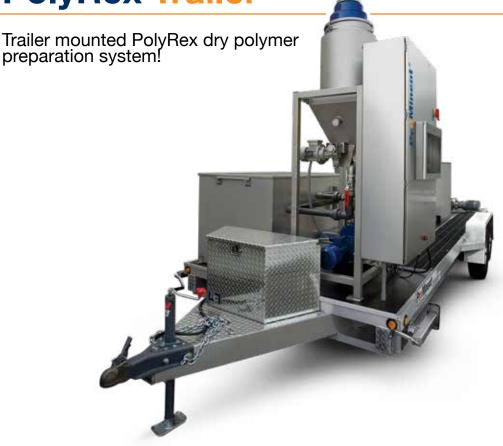
**ProMinent's** trailer mounted PolyRex dry polymer preparation system is fully integrated with everything needed for a successful on-site trial. System utilizes ProMinent's proven Optimo high energy mixer for dry polymer wetting followed by low energy mixing in the maturation tanks. Efficient preparation of dry polymer improves your process and saves operational costs.
