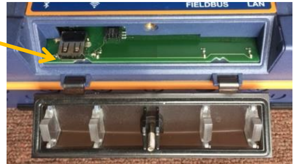
Figure 67 USB Access Door Closed [Top] and Open [Bottom]
