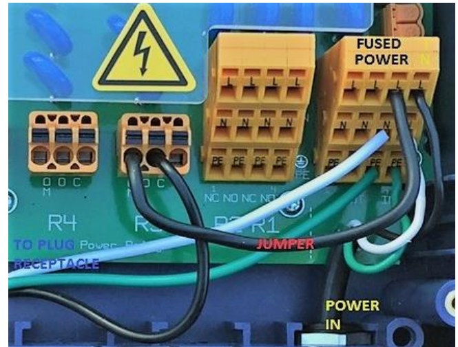
Figure 25 Wiring R3 using on-board fused power
