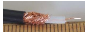
Figure 50B Coax cable preparation with black conductive sleeve removed
