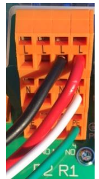
Figure 24 R1 MOV Wiring example
