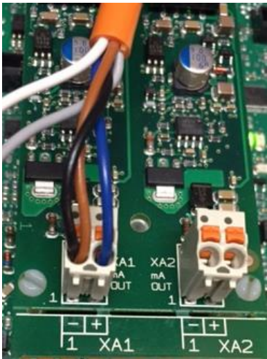
Figure 62 Dual mA Output with ProMinent Universal Control Cable on output 1.
