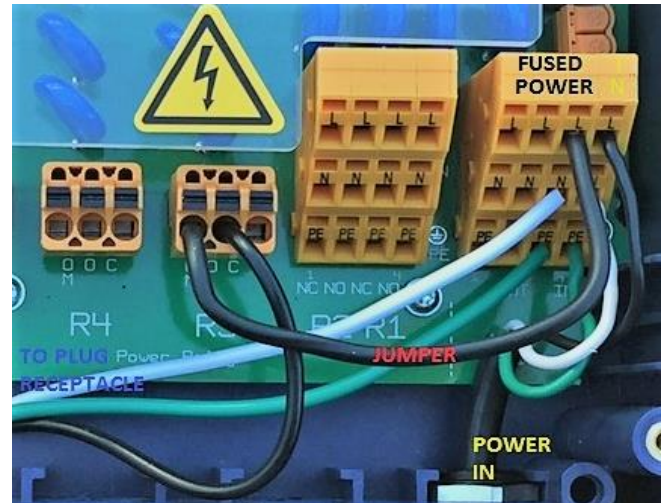
Figure 25 Wiring R3 using on-board fused power
