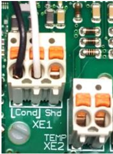
Figure 41 Two Wire Boiler Probe on XE1
