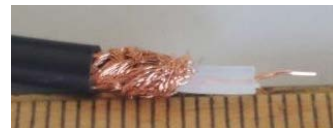
Figure 44B Coax cable preparation with black conductive sleeve removed
