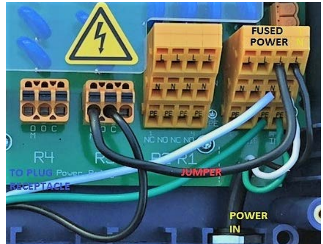
Figure 25 Wiring R3 using on-board fused power
