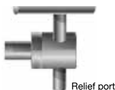
Backpressure valve on tee for pressure relief
