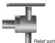
Backpressure valve on tee for pressure relief
