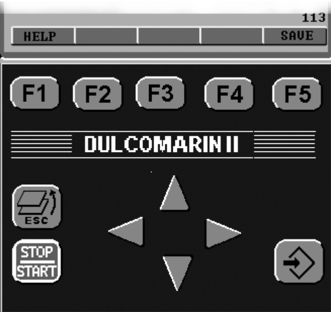
Fig. 5: Example for the allocation of function keys
