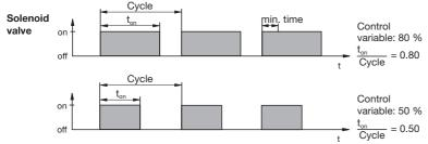
The switching time of the DULCOMETER® D1C (solenoid valve) depends on the actuating variable and the "min. time" (smallest permitted operating factor of the connected device). The actuating variable determines the ratio t<sub>or</sub>/cycle and thus the switching times (see fig. above).
