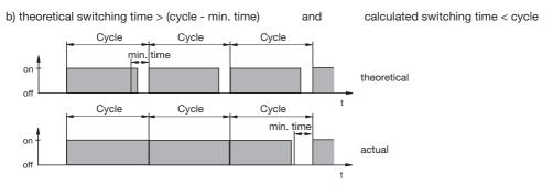
The DULCOMETER® D1C does not deactivate for a certain number of cycles until the differences between cycle and theoretical switching time exceed the "min. time".
