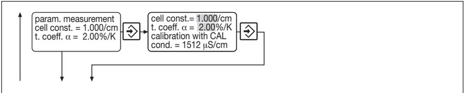
In “Parameter Measurement“ you can enter the cell constant or the temperature coefficient  $\alpha$  of your sample water.
