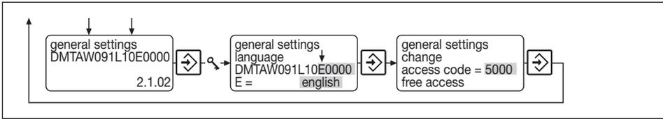
In the input menu “General Settings“ you can adapt the DMT to your special process requirement and activate an access code.
