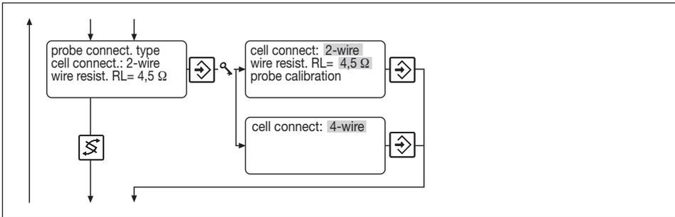
In Setting of “Conductivity Probe Connection“ you can select the connection type of the probe (2-wire or 4-wire connection)
