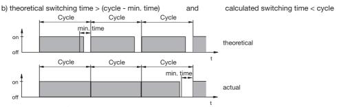
The DULCOMETER® D1C does not deactivate for a certain number of cycles until the differences between cycle and theoretical switching time exceed the "min. time".
