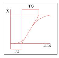
TU is influenced by the distance between the metering point and the point where the measuring water is extracted, the length of the measure water line and the velocity of flow. These factors cause a certain time to pass until the Chlorine change is registered at the controller.
