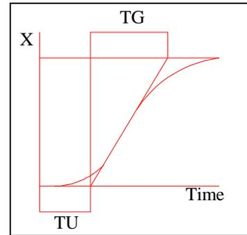
TU is influenced by the distance between the metering point and the point where the measuring water is extracted, the length of the measure water line and the velocity of flow. These factors cause a certain time to pass until the RH change is registered at the controller.
