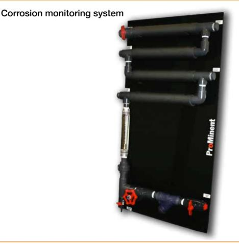
**ProMinent**<sup>®</sup> introduces a new **Corrosion Coupon Rack** designed for monitoring corrosion in cooling towers and boiler applications. The pre-engineered system is mounted on a backplane with 1" PVC piping. Includes visual inspection of coupons using clear PVC piping.
