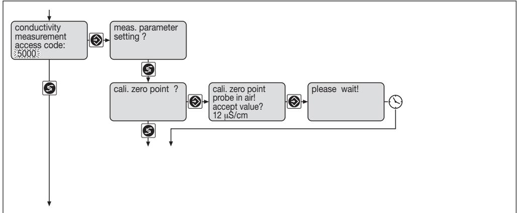
In order to determine the precise zero point (ZP) for the sensor, hold the sensor in the air – in the second menu item, the DULCOMETER® D1C displays the conductivity measured, without zero-point correction. If the value is constant, press the Enter key.
