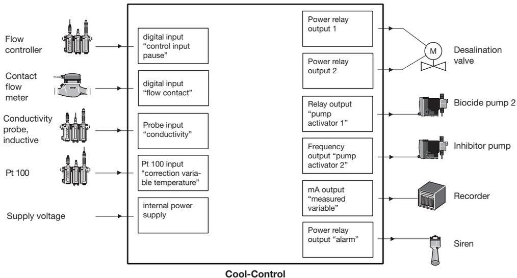
Fig. 2: Inputs/outputs for "power drive" "S"
