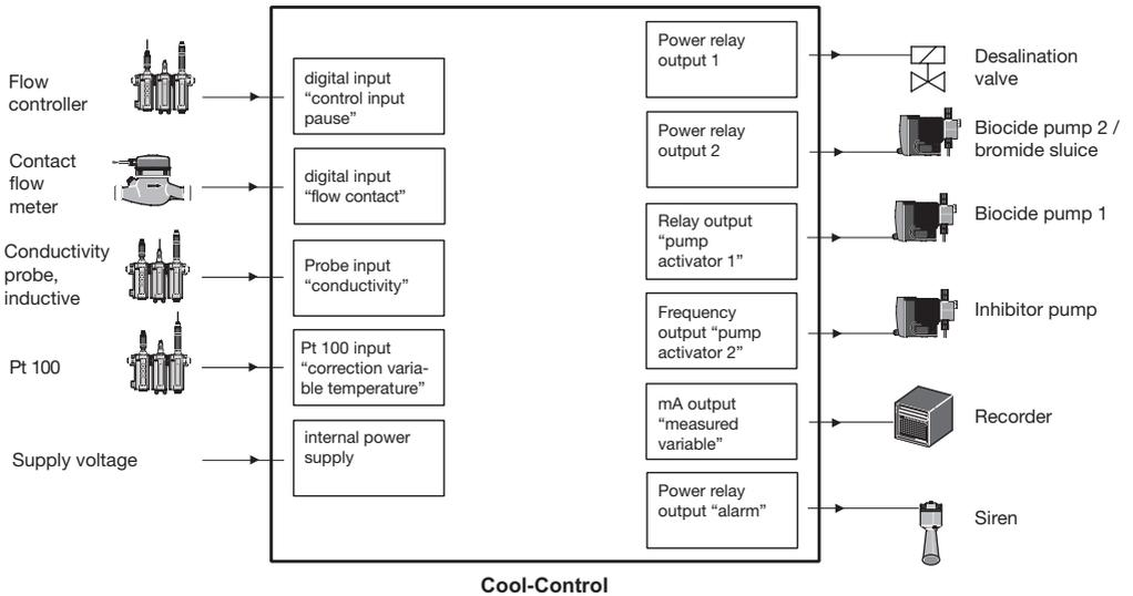
Fig. 1: Inputs/outputs for “Power drive” “G”
