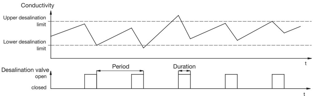
If the conductivity probe fails, the cooling tower can continue to be operated in emergency mode. The Cool-Control then carries out desalination independently of the conductivity probe at preset emergency mode intervals and for preset periods.
