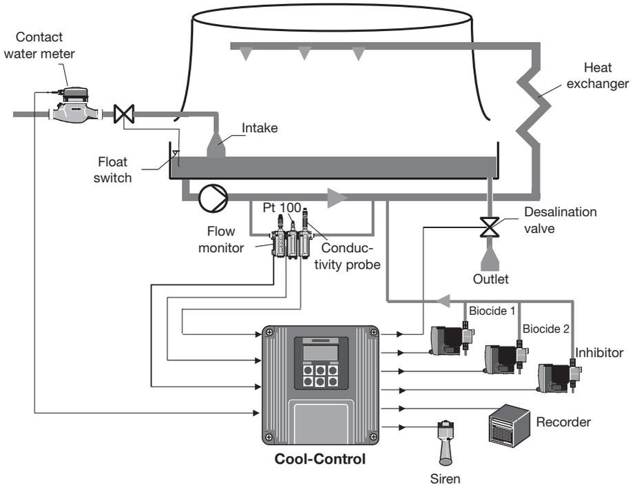
The water which evaporates from the cooling tower is replenished via the intake. The water level is kept constant by an independent float switch. The result of these processes is to increase the salt in the recirculating water. Therefore the desalination valve is opened at preset intervals to reduce the salt content. The resulting water loss is supplemented by the intake.
