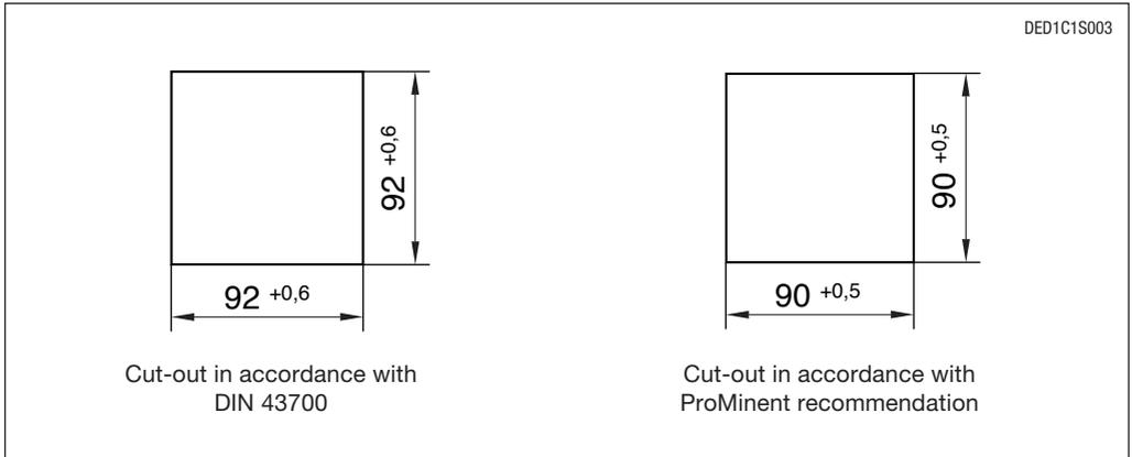
We recommend a smaller cut-out. The device is held in place better (less lateral play) and the seal is compressed evenly.
