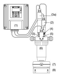
PAA measuring system in wall-mounted setup, with automatic temperature correction:
