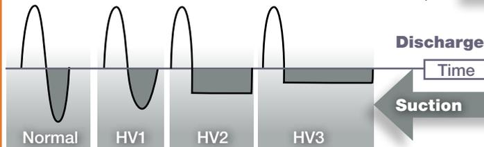
For prevention of cavitation, aggravation of off-gassing and pumping higher viscosity chemicals.
