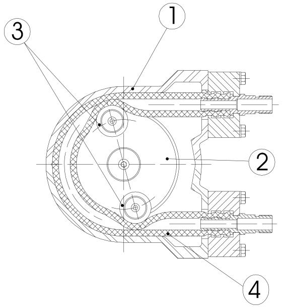
The outer casing (1) terminates with threading connectors. Inside the casing are found the rotor (2), completed with two rollers (3). As this is revolving it compresses the reinforced tube (4) and in this way generates a pumping action. A change in the direction of rotation will give rise to a change in direction of the pumped fluid.
