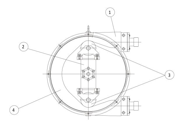
The outer casing (1) terminates with threaded connections. Inside the casing are found the rotor (2), complete with two rollers (3). As the rotor turns, the rollers compress the reinforced hose/tube (4), trapping a volume of fluid and forcing it out through the discharge. A change in the direction of rotation will give rise to a change in direction of the pumped fluid.
