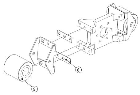
The shims are installed from factory to work at the operating conditions indicated in the application proposal, and according to the following table:
