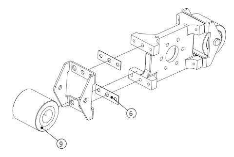
The shims are installed from factory to work at the work conditions indicated (in function of the speed and the work pressure), and following the next tables:
