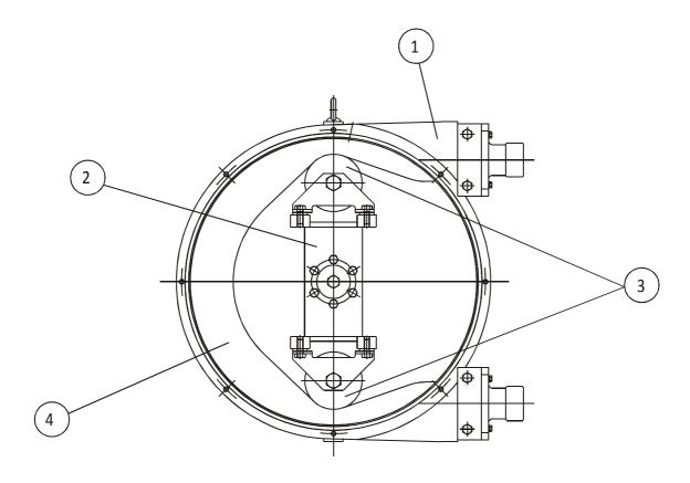
The outer casing (1) terminates with threaded connections. Inside the casing are found the rotor (2), completed with two rollers (3). As this is revolving it compresses the reinforced tube (4) and in this way generates a pumping action. A change in the direction of rotation will give rise to a change in direction of the pumped fluid.
