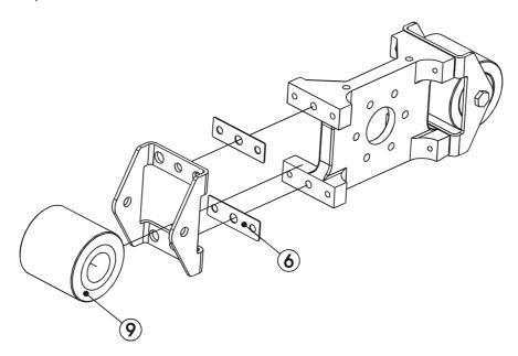
The shims are installed from factory to work at the work conditions indicated (in function of the speed and the work pressure), and following the next tables:
