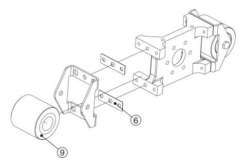
The shims are installed from factory to work at the work conditions indicated (in function of the speed and the work pressure), and following the next tables: DFC70 (number of shims of 1 mm.)
