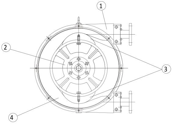
The outer casing (1) terminates with clamp connectors PN-16. Inside the casing are found the rotor (2), completed with two rotor shoes (3). As this is revolving it compresses the reinforced tube (4) and in this way generates a pumping action. A change in the direction of rotation will give rise to a change in direction of the pumped fluid.
