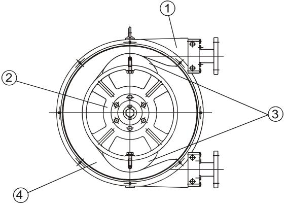
The outer casing (1) terminates with clamp connectors PN-16. Inside the casing are found the rotor (2), completed with two rotor shoes (3). As this is revolving it compresses the reinforced tube (4) and in this way generates a pumping action. A change in the direction of rotation will give rise to a change in direction of the pumped fluid.
