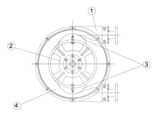
The outer casing (1) terminates with clamp connectors PN-16. Inside the casing are found the rotor (2), completed with two rotor shoes (4). As this is revolving it compresses the reinforced tube (3) and in this way generates a pumping action. A change in the direction of rotation will give rise to a change in direction of the pumped fluid.
