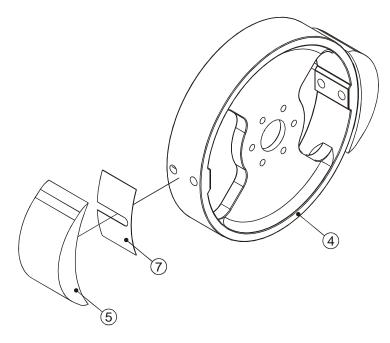
The shims are installed from factory to work at the work conditions indicated (in function of the speed and the work pressure), and following the next tables:
