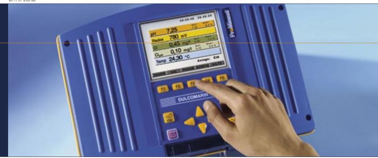
The Dulcometer® Disinfection Controller/Monitor and DULCO®-net technology are revolutionizing measuring, control and metering technology in public water systems. The decentralized modular concept with one single central unit controls sensors and actuators for up to 16 measurement locations.
