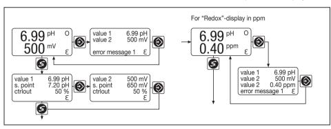
The device function can be monitored via permanent displays 1,
