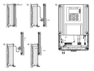
The following apertures can be used when wall-mounting:
