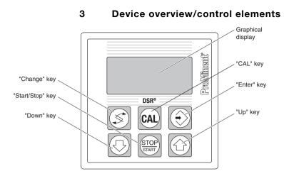
The DSR controller graphical display uses the following symbols:
