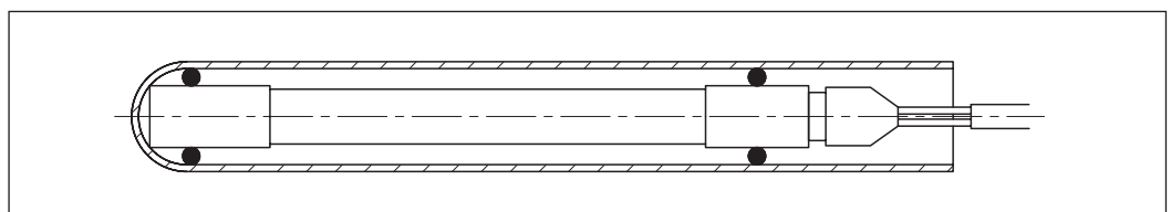
Figure 6: Lamp with O-rings to assist insertion into lamp protection tube
