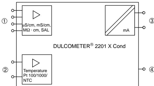
Fig. 6 System functions of DULCOMETER<sup>®</sup> 2201 X Cond
