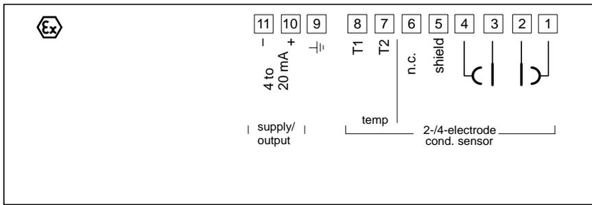
Fig. 7 Terminal assignment of DULCOMETER® 2201 X Cond
