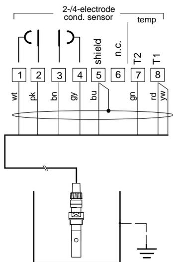
Fig. 8 Conductivity measurement with LF 604 2-electrode cell
