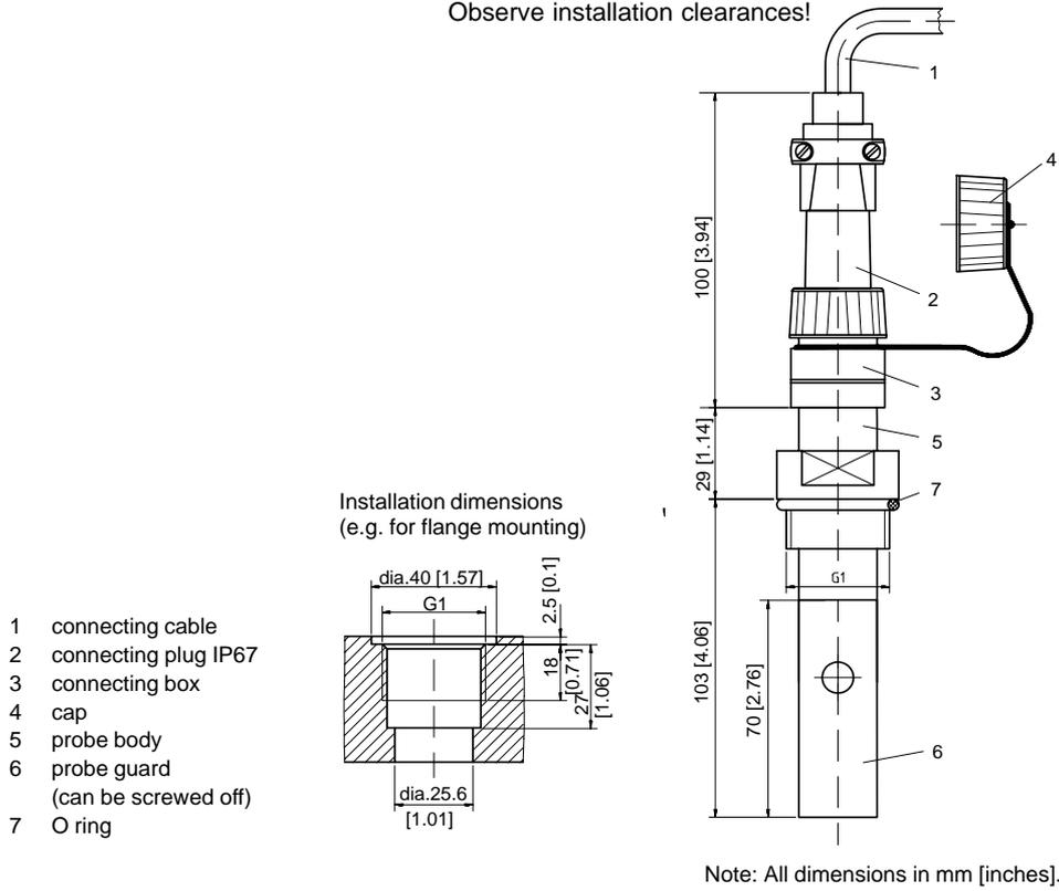
Fig. 11 Dimension drawing LF 604 2-electrode cell
