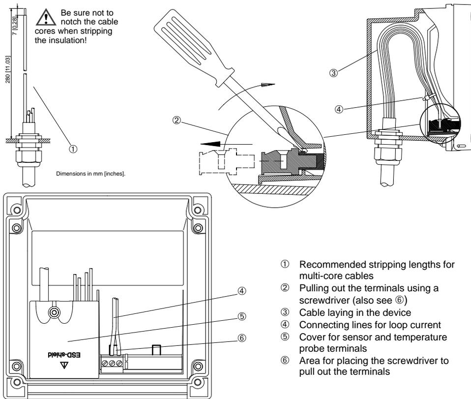
Fig. 5 Installation information DULCOMETER® 2201 X Cond
