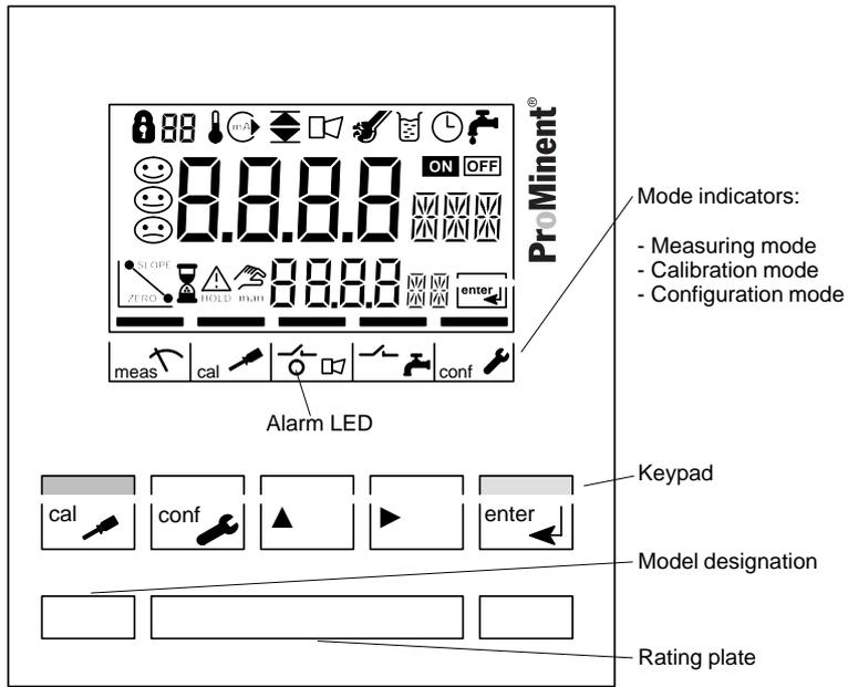
Fig. 9 Front view of DULCOMETER® 2201 X Cond
