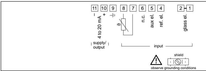
Fig. 7 Terminal assignment of DULCOMETER® 2201 X pH
