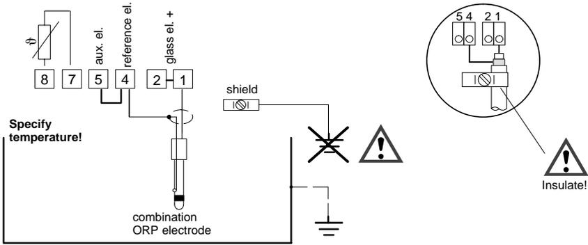
Fig. 17 ORP measurement with combination ORP electrode without temperature probe
