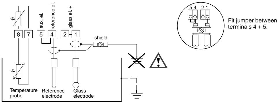
Fig. 10 pH measurement with separate glass and reference electrode and temperature probe, Sensocheck® limited to the glass electrode only
