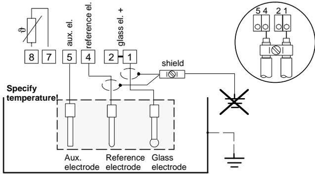
Fig. 15 pH measurement with separate glass, reference and aux. electrode without temperature probe, Sensocheck® for glass and reference electrode
