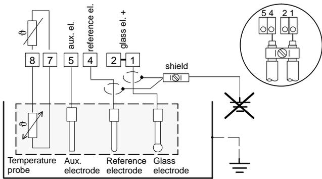
Fig. 14 pH measurement with separate glass, reference and aux. electrode and temperature probe, Sensocheck® for glass and reference electrode
