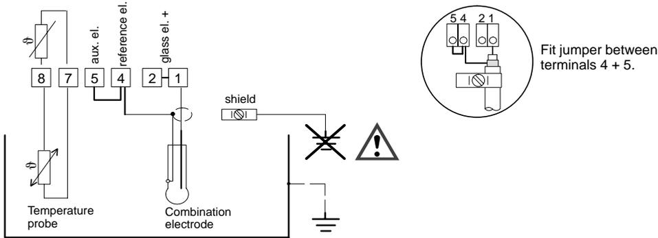
Fig. 8b pH measurement with combination electrode and temperature probe, Sensocheck® limited to the glass electrode only
