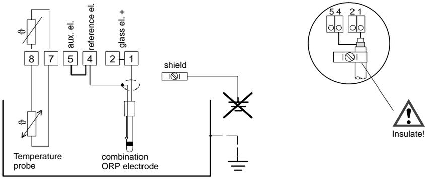
Fig. 16 ORP measurement with separate combination ORP electrode and temperature probe
