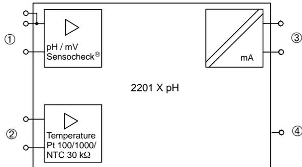
Fig. 6 System functions of DULCOMETER® 2201 X pH
