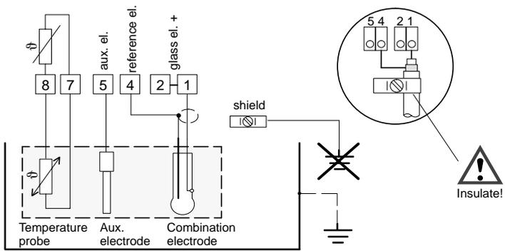
Fig. 12 pH measurement with combination and aux. electrode and temperature probe, Sensocheck® for glass and reference electrode
