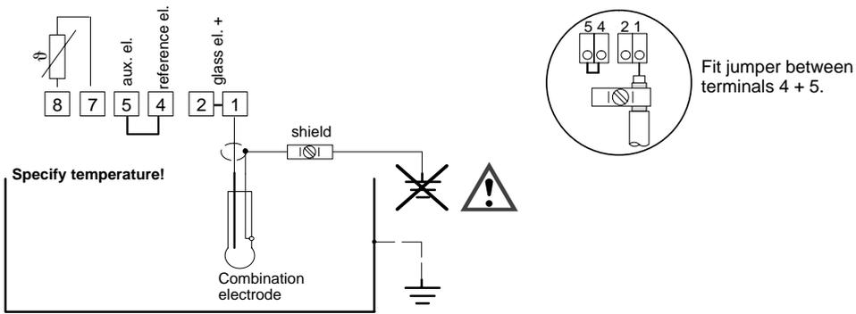
Fig. 9 pH measurement with combination electrode without temperature probe, Sensocheck® limited to the glass electrode only
