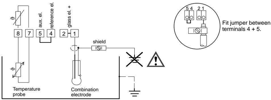
Fig. 8a pH measurement with combination electrode and temperature probe, Sensocheck® limited to the glass electrode only
