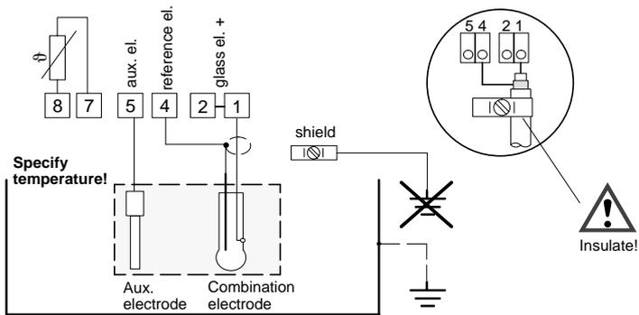
Fig. 13 pH measurement with combination and aux. electrode without temperature probe, Sensocheck® for glass and reference electrode
