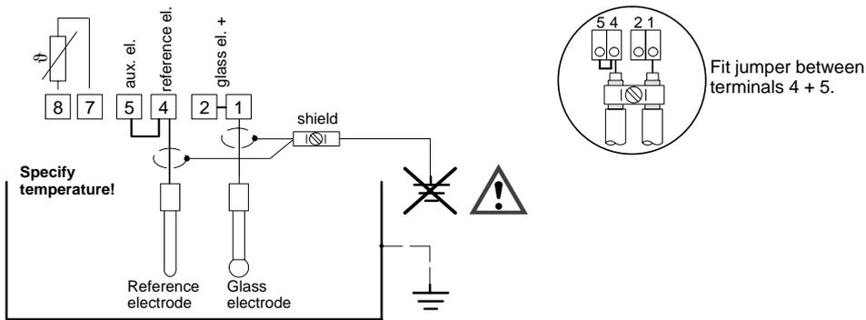
Fig. 11 pH measurement with separate glass and reference electrode without temperature probe, Sensocheck® limited to the glass electrode only
