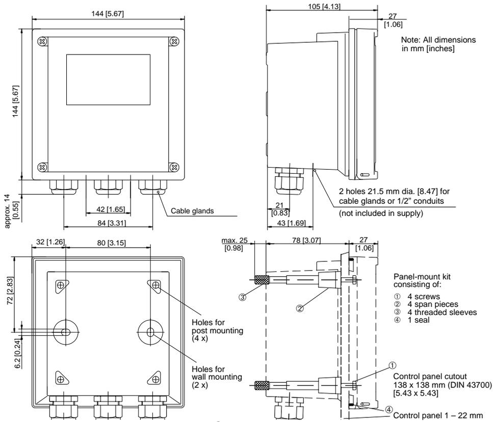
Fig. 2 Dimension drawing for DULCOMETER® 2201 X pH, mounting diagram and panel-mount kit (Order No. 1008708)
