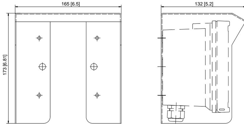
Fig. 4 Protective hood (Order No. 1008709) for wall and pipe mounting
