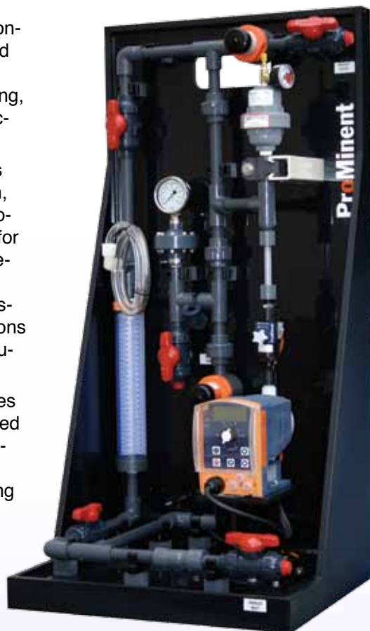
Standard SS1 single pump system with ProMinent metering pump, integrated calibration column, pressure relief valve, backpressure valve, pulsation dampener, flow monitor and pressure gauge.
