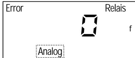
In order to acknowledge the error message at least 4 mA must be applied at the signal current input, after this the pump starts again independently and the error display "Error" and the flashing "Analog" go off.
