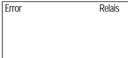
Display in the event of an automatic pump stop as timer relay
