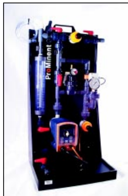
Standard single dosing unit (S-1) with a gamma/L metering pump mounted on a UV protected Polyethylene (PE) stand.
