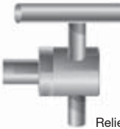
Backpressure valve on tee for pressure relief
