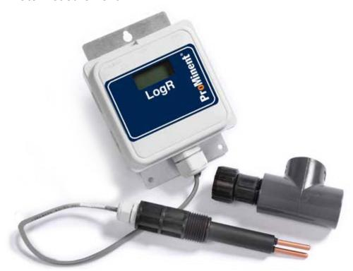
The **ProMinent® LogR** is a single channel corrosion rate monitor using **Linear Polarization Resistance (LPR)** to measure the corrosion rate of metals in cooling water treatment applications. Weight loss coupon results can take weeks or months. With the **LogR**, a reading is taken every 2.5 minutes giving accurate corrosion rates instantly. Select from **carbon steel**, **copper or admiralty** sensors.
