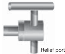
Backpressure valve on tee for pressure relief
